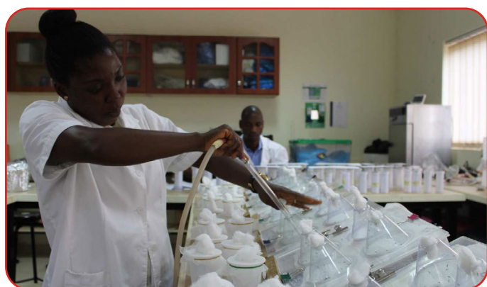
Figure 6. Bioefficacy testing of PermaNet® at Vestergaard-NMIMR Vector Labs in Accra, Ghana following WHO guidelines
