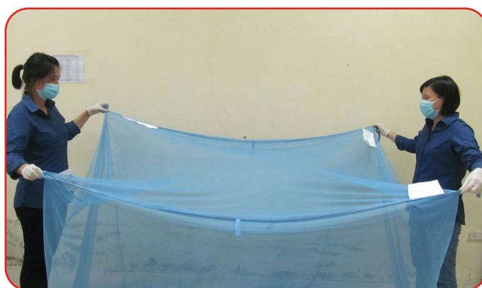
Figure 7. Inspection for workmanship and appearance in the Acceptance Testing and Inspection scheme
