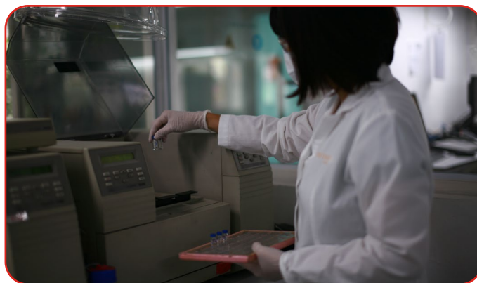
Figure 3. Analysing deltamethrin content with High Performance Liquid Chromatograph in Vestergaard Vector Control Laboratory in Hanoi, Vietnam
