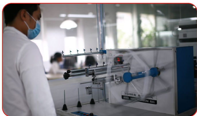
Figure 4. Measuring denier of yarn in Vestergaard Vector Control Laboratory in Hanoi, Vietnam to ensure only the highest quality yarn is used for PermaNet® LLINs production
