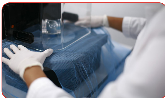
Figure 5. Measuring bursting strength of finished net in the Acceptance Testing and Inspection scheme
