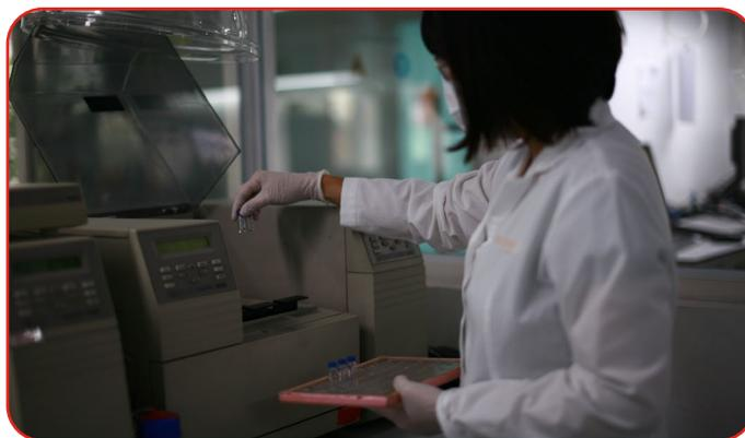
**Figure 3.** Analysing deltamethrin content with High Performance Liquid Chromatograph in Vestergaard Vector Control Laboratory in Hanoi, Vietnam
